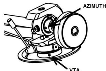
With the aid of a good magnifying glass adjust the needle until it is vertical in the groove (i.e. perpendicular to the record's surface). Ideally this should correspond to the top surface of the cartridge body being parallel to the record surface, but in practice this is often not the case.
