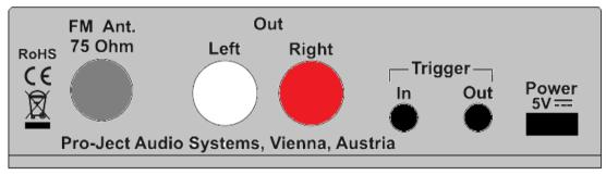
Make all connections whilst the tuner is disconnected from the power supply. Take care to connect the left and right channels correctly. The right channel is usually marked red, the left channel black or white.
