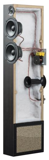
The 19mm thick cabinet is perfectly made to block any sound-leakage. The interior of the loudspeakers is kept to be as simple as possible. The PCB-less design guarantees an undisturbed signal-path to the drivers.
