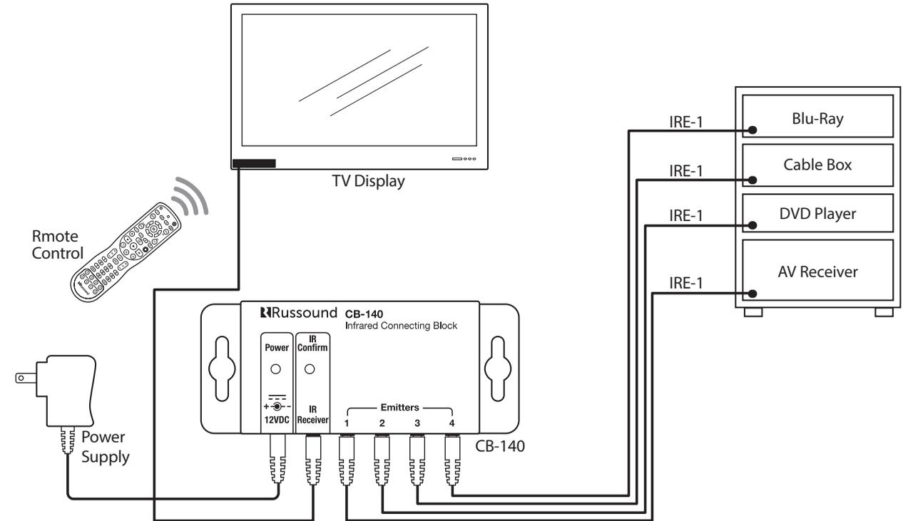
All of the wires from the emitters and the receiver connect easily with color-coded connectors into the CB-140 connecting block.
