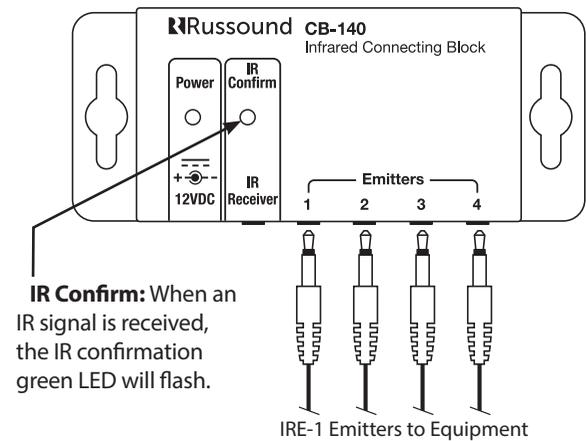
**IR Confirm:** When an IR signal is received, the IR confirmation green LED will flash.
