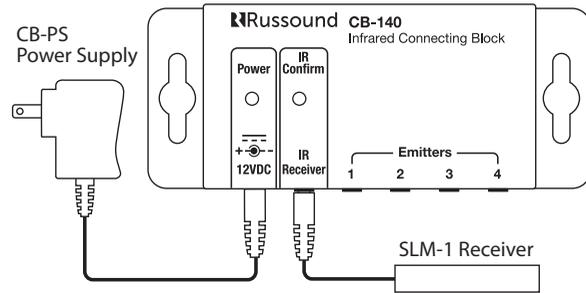
**Emitter Outputs:** Connect up to 4 emitters to the emitter jacks labeled 1-4 (green connectors).
