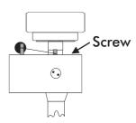
With the aid of a good magnifying glass adjust the needle until it is vertical in the groove (i.e. perpendicular to the record's surface). Ideally this should correspond to the top surface of the cartridge body being parallel to the record surface.
