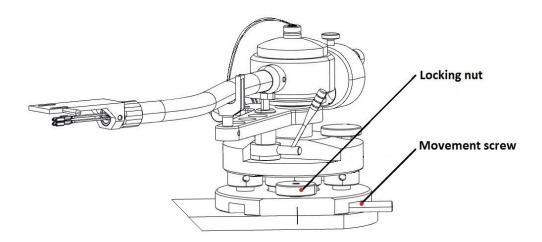
Loosen the locking nut allows a linear move of the tonearm. Adjust correct distance by using the scale. The correct mounting distance of 238 mm on the scale is valid only if the cartridge is in correct position in the headshell.
