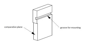
**Step 1:** Place the tool with groove to the headshell as shown.
