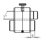
b) If the additional weight is placed unsymmetrically (as shown in the picture bellow, 12mm visible part from the rear side), it can balance cartridges with weight of **17 to 20 grams**.
