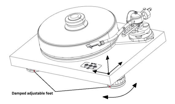
Three precision adjustable damped feet are mounted under the turntable for levelling the turntable. Once the turntable is in final position, put the supplied spirit level on the chassis, and then level the turntable by screwing or unscrewing the feet as needed. It is advisable to check level from several positions on the chassis.
