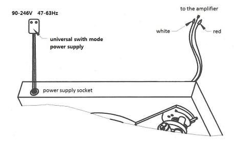
The turntable is supplied with the universal power supply (90-246V AC) with 3 exchangeable sockets adapters suitable for all countries. Select the correct adapter for your country and insert the adapter to the exchangeable part of the power supply.
