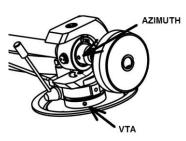
With the aid of a good magnifying glass adjust the needle until it is vertical in the groove (i.e. perpendicular to the record's surface). Ideally this should correspond to the top surface of the cartridge body being parallel to the record surface, but in practice this is often not the case.
